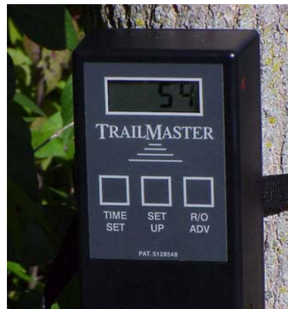
Figure 3: Infrared Trail Counter Receiver Unit
