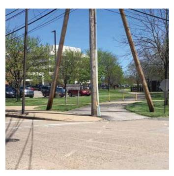
The utility pole in the center of the ramp at 2nd Street should be relocated. | Photo courtesy RTC
