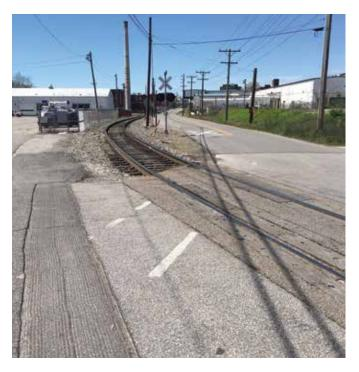
The railroad crossing at Depot Street renders the bike lane unusable. The roadway should be widened where possible to ensure clear passing width for all users. |
