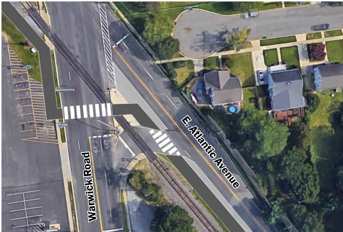
A schematic layout of potential changes to the East Atlantic Avenue & Warwick Road intersection to allow for trail construction.
