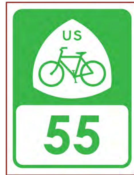
The newest version of USBR signage granted interim approval by the FHWA. Source: Halff Associates (Derived from MUTCD, 2009)
