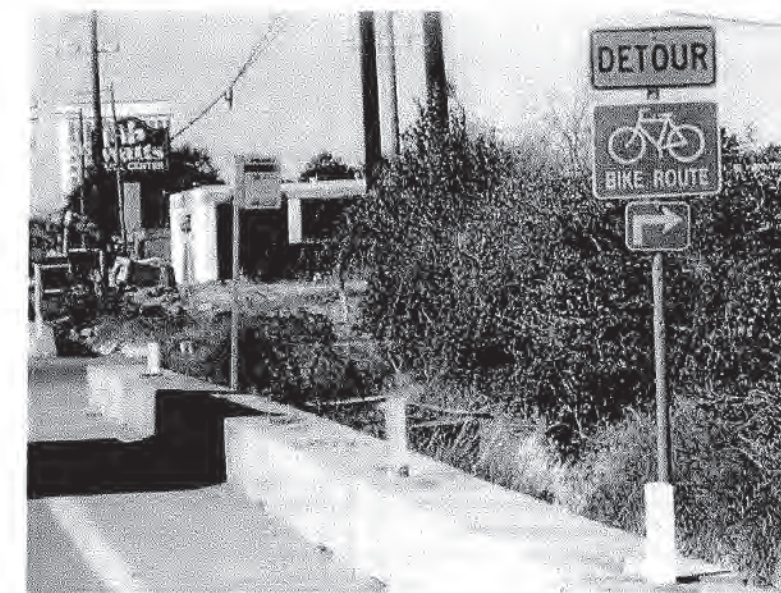
Example of detour sign placed on a bike route sign.
