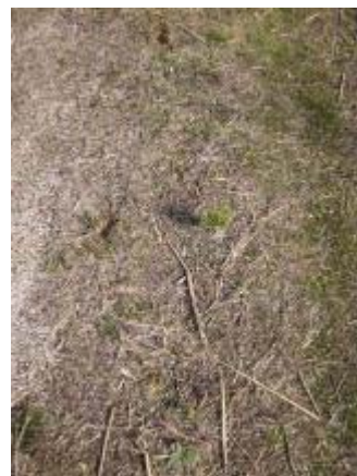
Photo 54 Soiltac Liquid Topical trail segment remained soft through the final testing. November 2, 2011.
