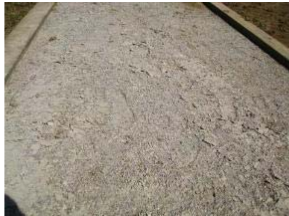
Photo 46 Soiltac Liquid Topical trail segment became soft under foot. March 13, 2008.
