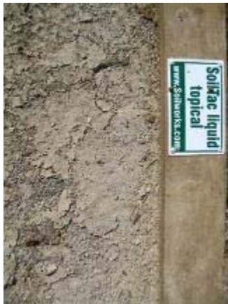
Photo 45 Soiltac Liquid Topical trail segment showed change after a heavy rainfall. March 13, 2008.
