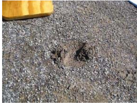
Photo 82 Stabilizer trail segment shows indentation from surface testing. March 13, 2008.
