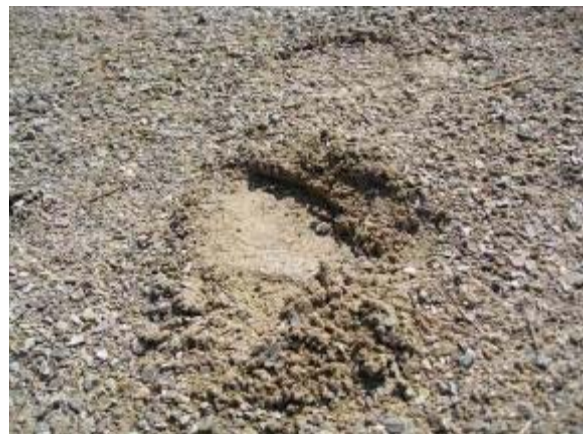
Photo 138 Quarter Inch Minus Limestone trail segment would only firm up after extended periods of no moisture. March 17, 2009.
