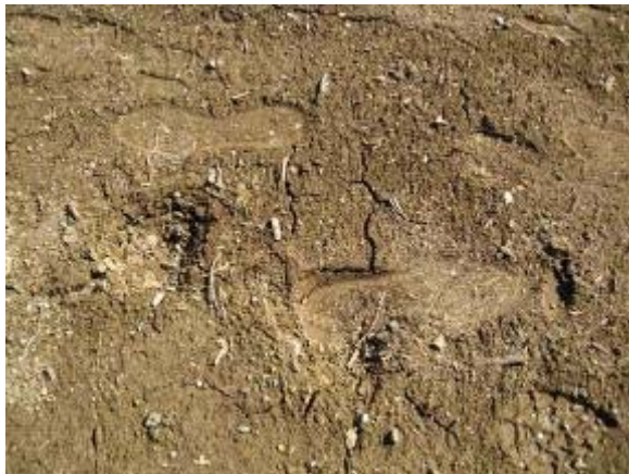
Photo 116 Polypavement trail segment would remain soft underfoot. March 13, 2008.
