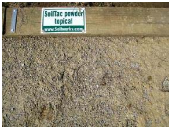
Photo 21 Soiltac Powder Topical has formed a solid paper-thin layer after a heavy rainfall. March 13, 2008.
