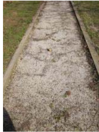
Photo 68 Soiltac Liquid Mix-In performed better than its topical application counterpart. November 2, 2011.
