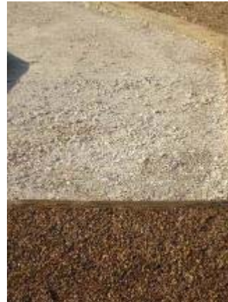
Photo 91 StaLok is applied to a base of 3 inches of compacted native soil. June 21, 2007.
