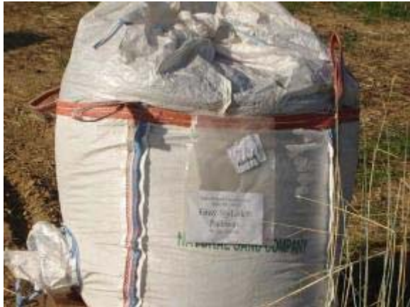
Photo 90 StaLok arrives pre-mixed with ¼ inch minus aggregate. June 21, 2007.
