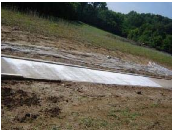
Photo 20 Soiltac Powder Topical has a penetration of 1/8 inch. June 27, 2007.
