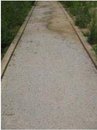
Photo 49 Soiltac Liquid Topical trail segment remained soft where water had pooled. June 12, 2008.
