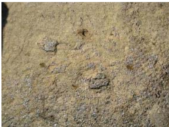
Photo 22 Soiltac Powder Topical was soft under foot and showed footprints. March 13, 2008.
