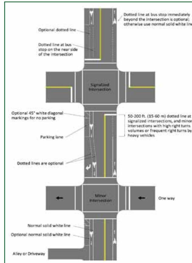
Figure 7.7. **Bike Lane Pavement Markings.**
