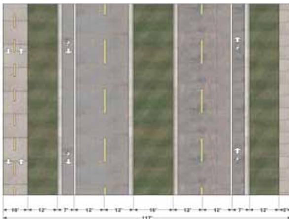
Figure 7.11. (left) **Four-lane divided section with sidepath**
