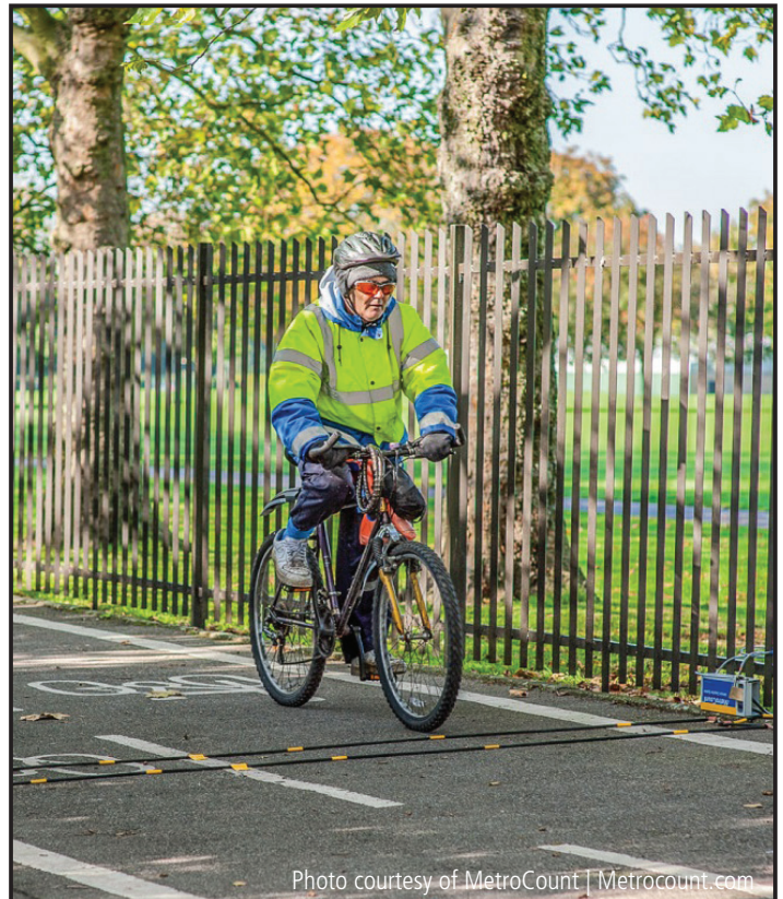
A biker passes a short-duration count station with a passive infrared counter and pneumatic tubes.
