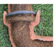
(Left) Tree roots can clog pipes, causing drainage problems and local flooding.
