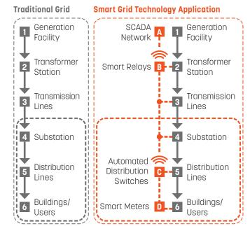
(Above) Smart Grids can benefit each stage of the electricity generation, transmission, and distribution cycle. A disruption at any stage can cause cascading power outages throughout a traditional grid system while in a Smart Grid Network, communication technologies allow the grid to share information across each node.
