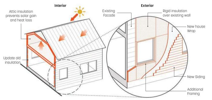
External insulation is an option for cladding over the existing facade where interior retrofit may be too invasive
